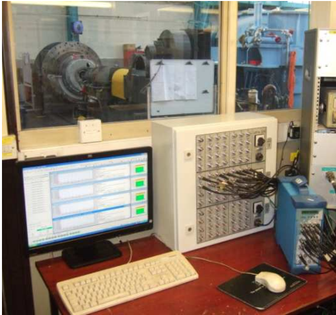
Fig. 1: The OROS OR36 and NVGate in use at our end of line production test facility
